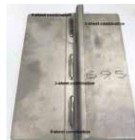
*Figure 1: Laser welded 3 ply titanium skin lap joint (Images courtesy of TWI and IPG Photonics) - laser seam stepper welding.*
