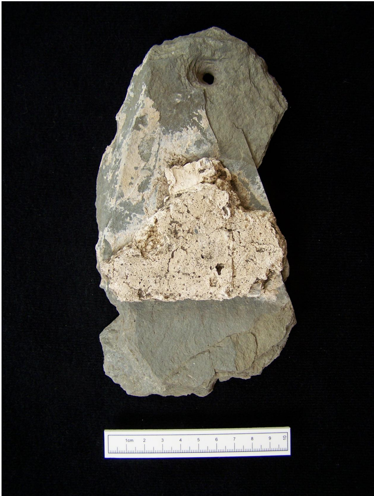
Plate 19: The back of a roofing 'slate' upon which a longitudinal seam is preserved on the surface of the mortar bed (Small Find No.1040). This seam was formed by the mortar squeezing up between the adjoining edges of the two 'slates' laid on to the mortar bed. That it approximately lines up with the centrally-placed fixing hole indicates that the overlying 'slates' formed a near 50% overlap. Scale 10 centimetres.
