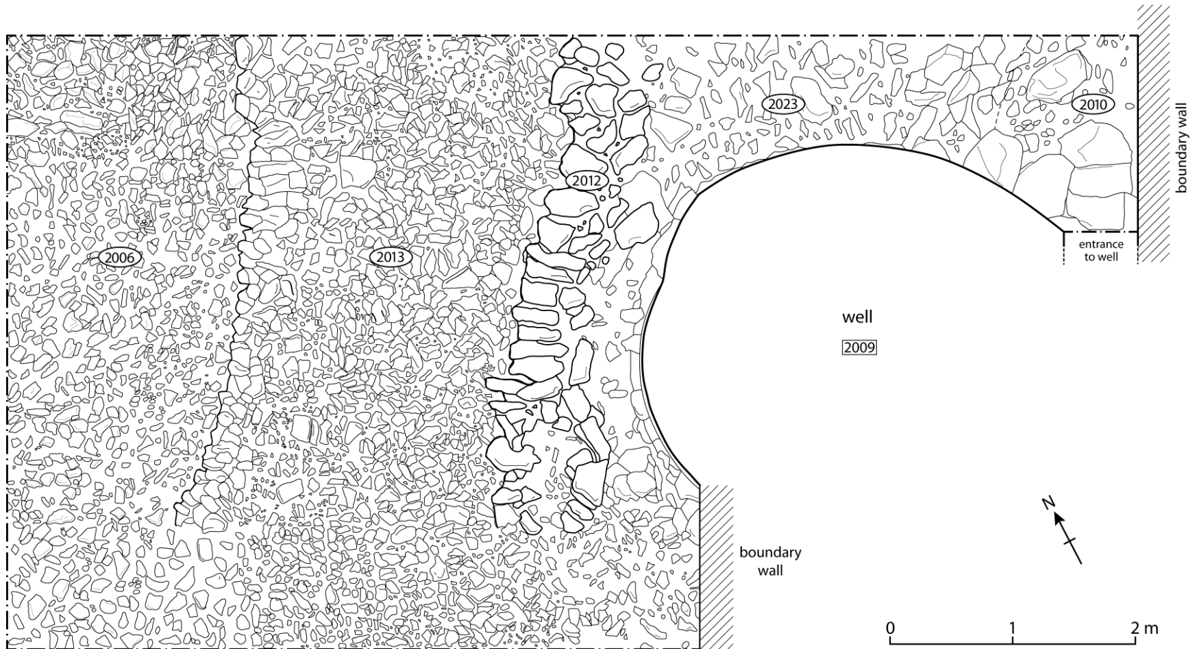
Figure 19 Trench 2: Plan showing the metallised roadway and cobbled path (scale 1: 20cm).
