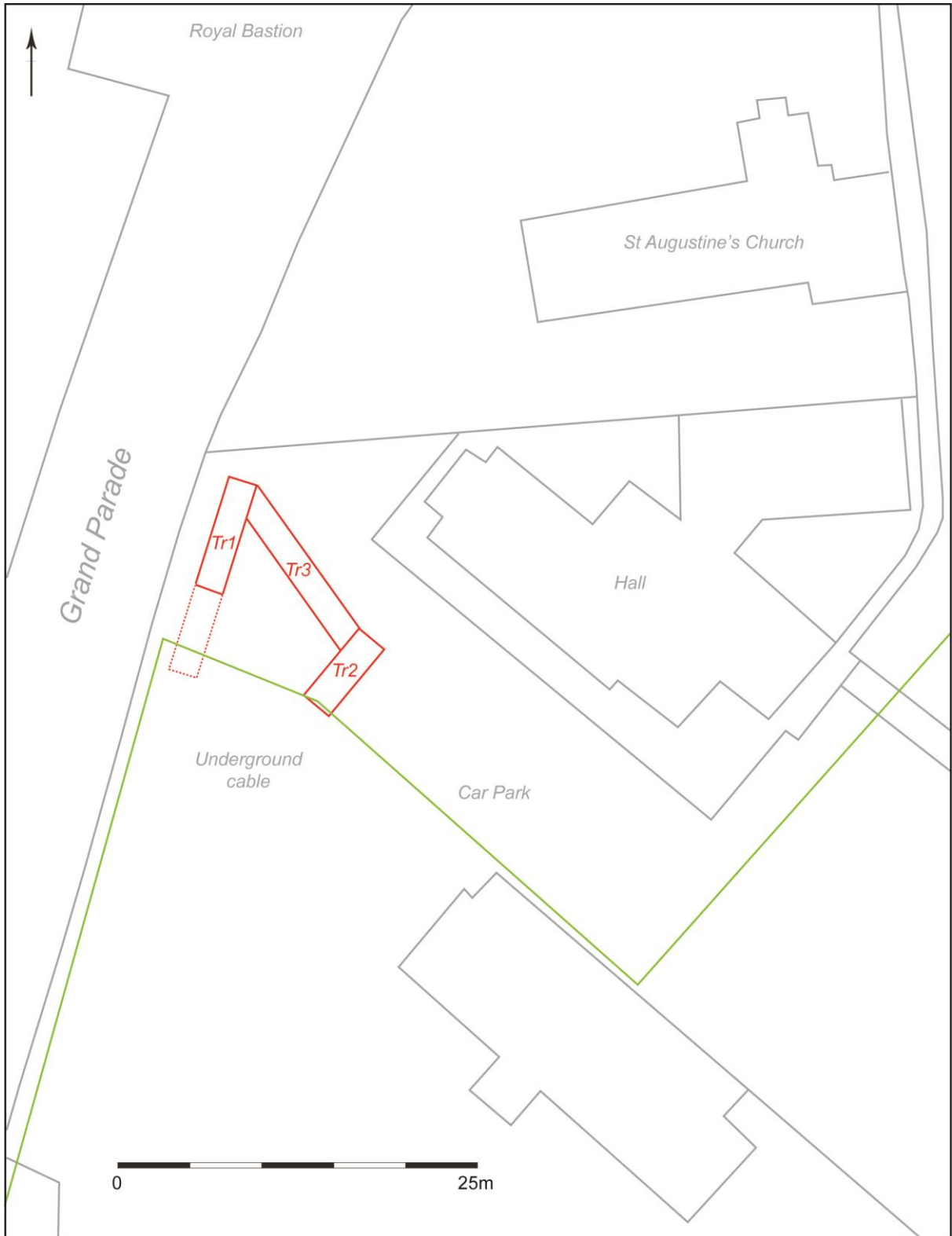
Figure 15 Location of the evaluation trenches (image prepared by Sapphire Mussen) with NIE cables (green line) also shown. The NIE line traversing the car-park from Grand Parade to Bishop Street within follows the line of a former wall, removed sometime post-2005 (wall marked on the 2005 OSNI map of the city).
