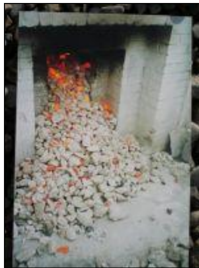
Figure 13: Example of burnt lime, www.buildinglimesforumireland.com
